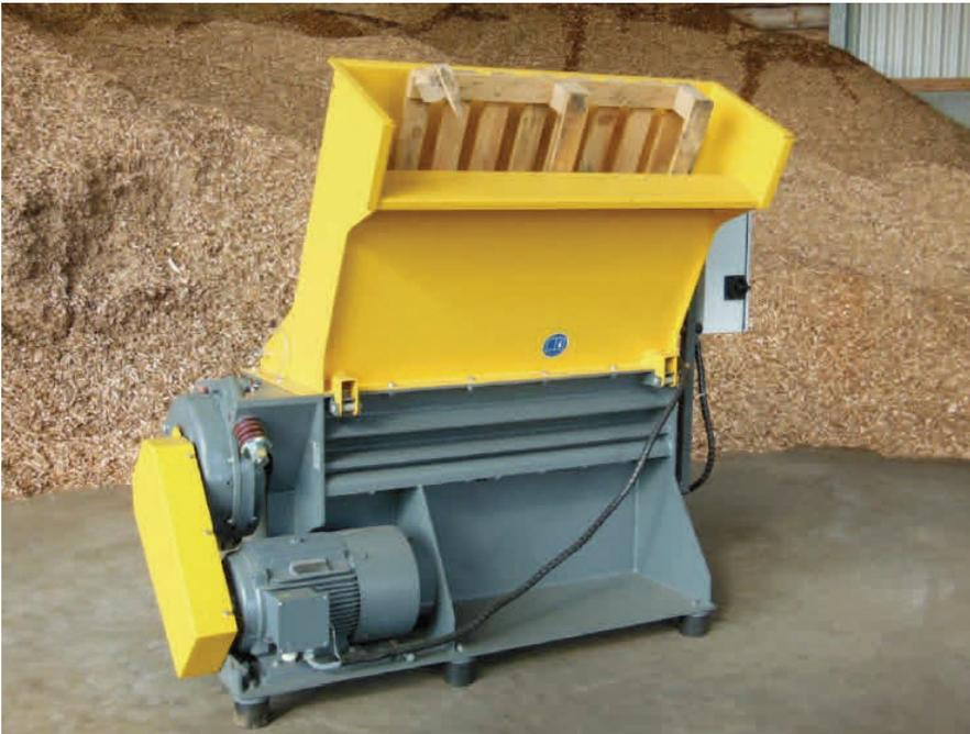
The chipper has a reversible counter knife and 36 rotating cutting blades, which are intended for two time utilization.
